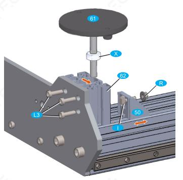
To mount the adjustable feet, the respective corner bracket must be unscrewed, moved and reconnected to profile 10
