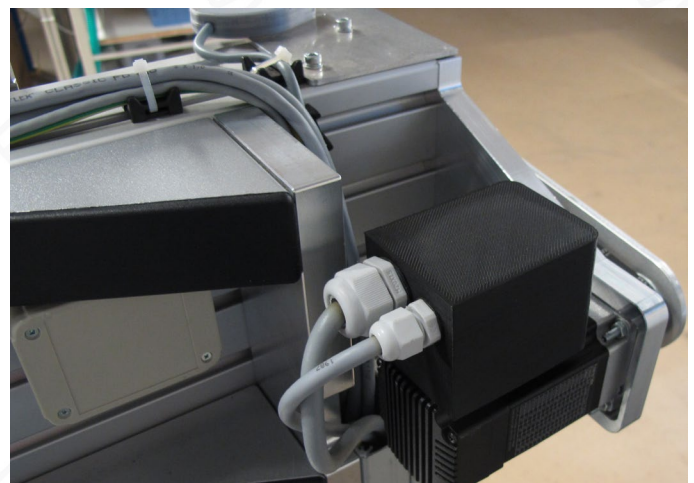
Fig. 7: The cover protects against dust and chips.
