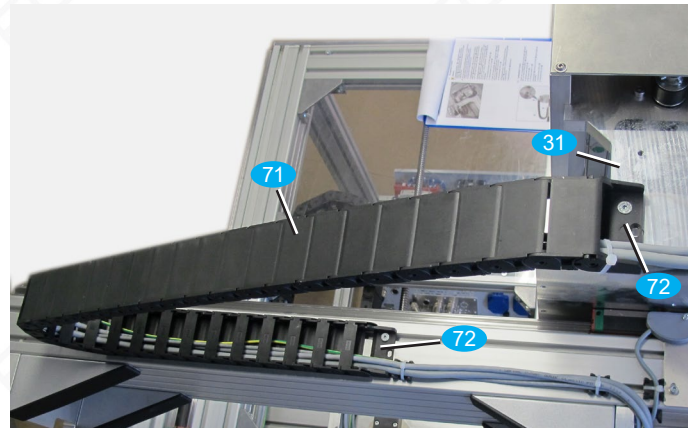
Fig. 2: Cable routing through the Y-axis drag chain.
