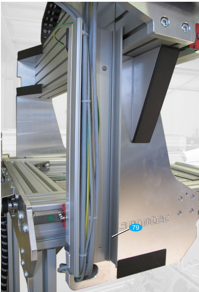
Fig. 3: Cable routing through cable duct. The cover is missing for a better overview.
