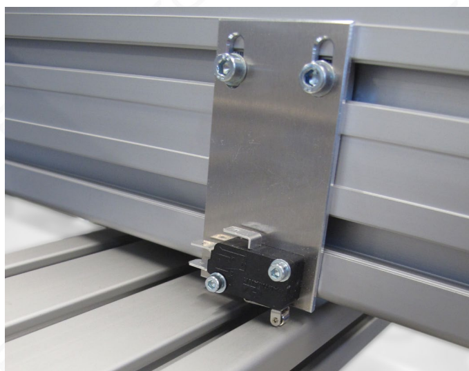
Fig. 7: Triggering of the reference switch by the beam
