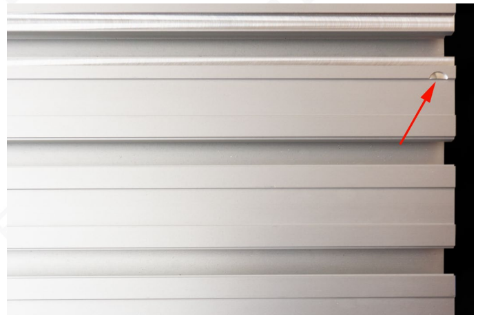
Fig. 9: Marking of the upper stop milling
