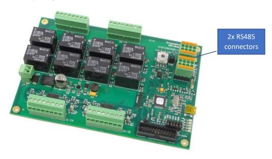
Please note, the last interface card that is daisy chained needs to have its termination resistors enabled. On the other boards this termination should be disabled.
