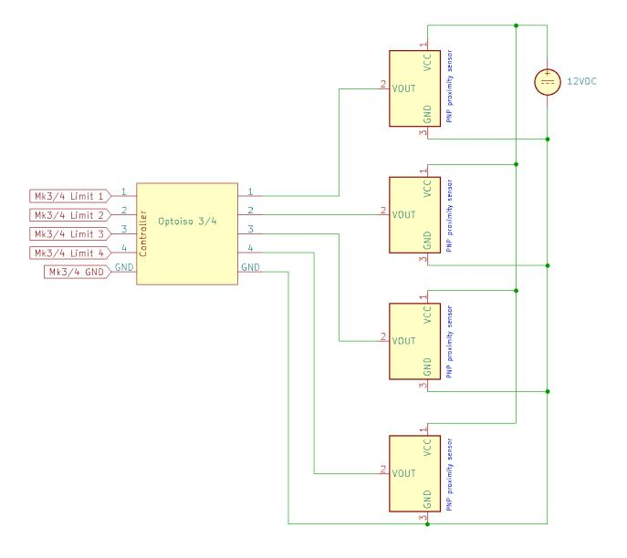
PNP proximity sensor 12 VDC power supply
