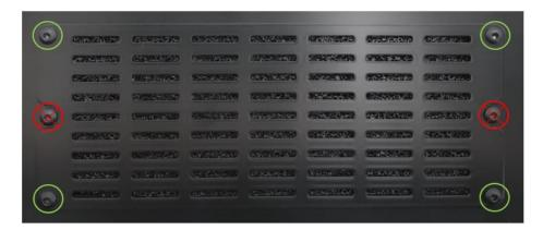
The filter must be removed for cleaning and then cleaned with a vacuum cleaner or compressed air gun, for example. After cleaning, the filter must be reinserted, and the fan grille screwed on finger tight. The Xcool must not be operated without the filter and the protective grille of the fan.
