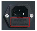
The old fuse must be removed and replaced with a new one. The fuse compartment must then be reinserted until it clicks into place. The Xcool is ready for operation again.
