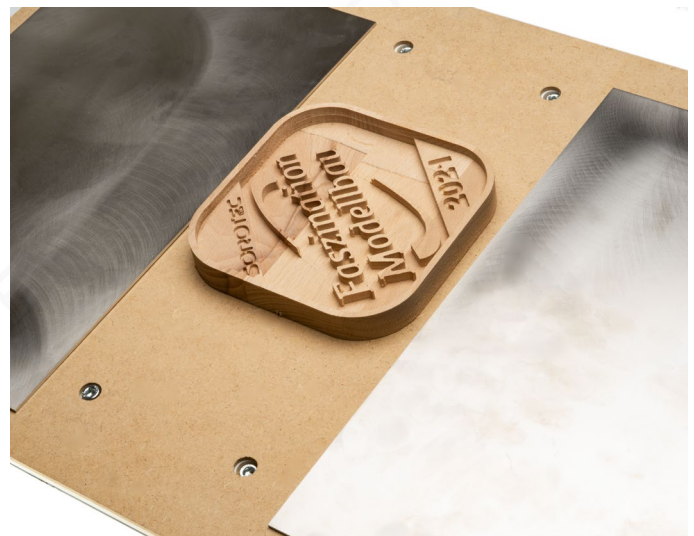
Fig. 4: Covering of unused areas, here as an example with sheet metal
