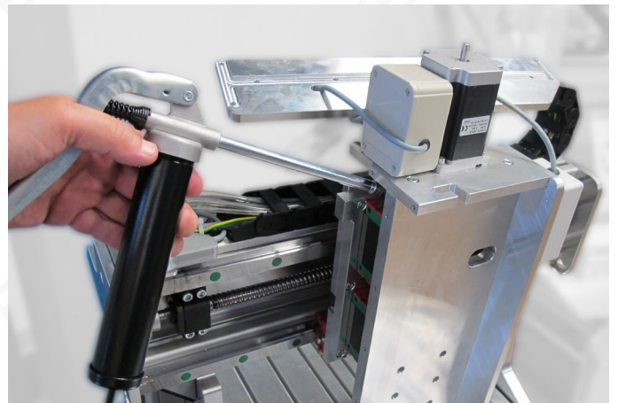
Fig. 9: Lubricating the left Z guides
