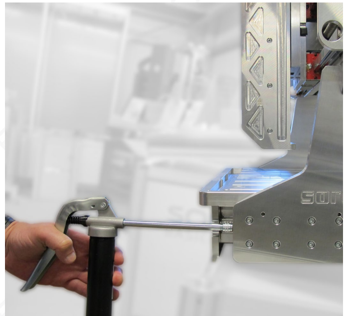
Fig. 1: Lubricating guide carriage X-axis
