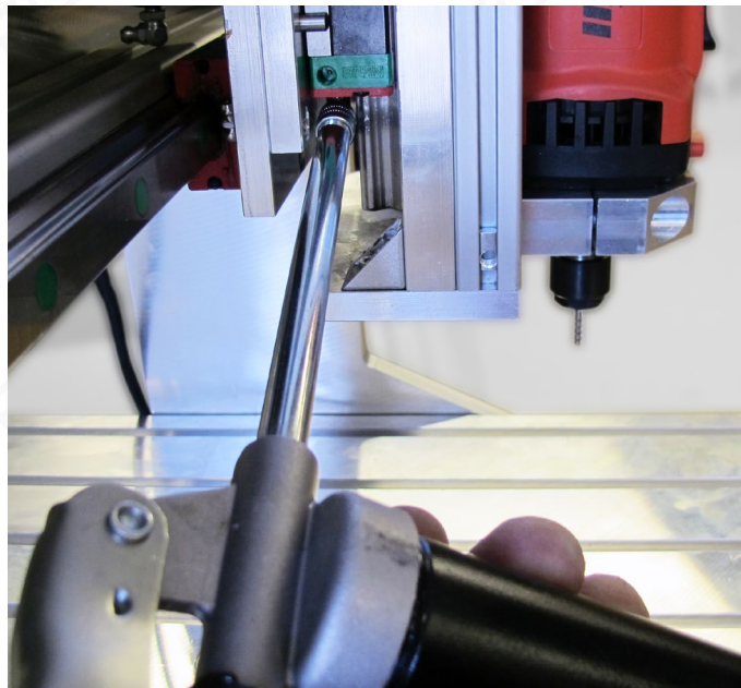
Fig. 48: Lubricating guide carriages Z-axis
