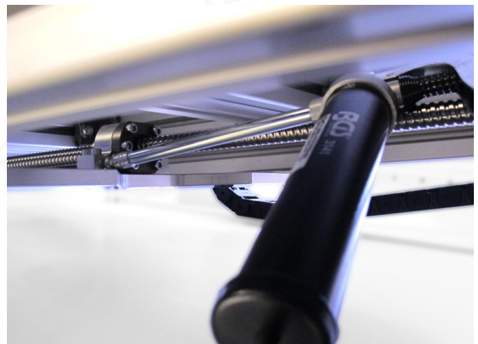
Fig. 45: Lubricating the X-spindle nut with the machine tilted forward
