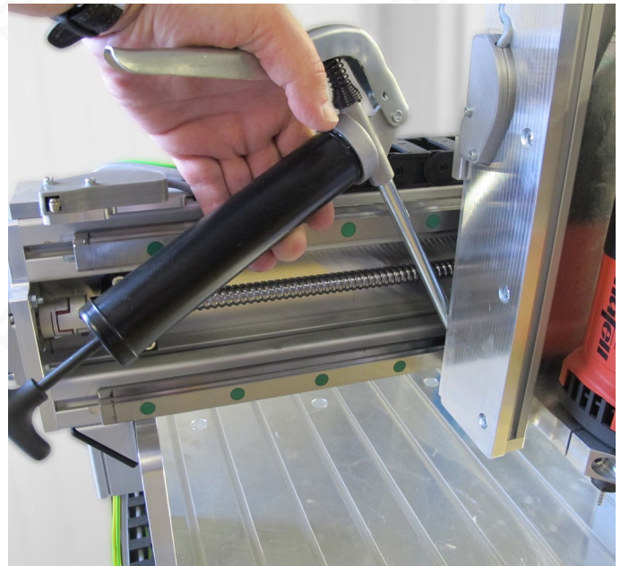
Fig. 46: Lubricating guide carriages Y-axis
