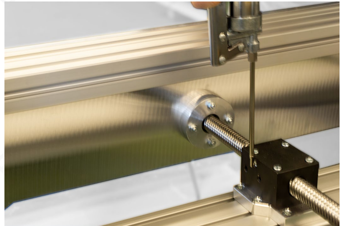
Fig. 3: Lubricating the center spindle from above
