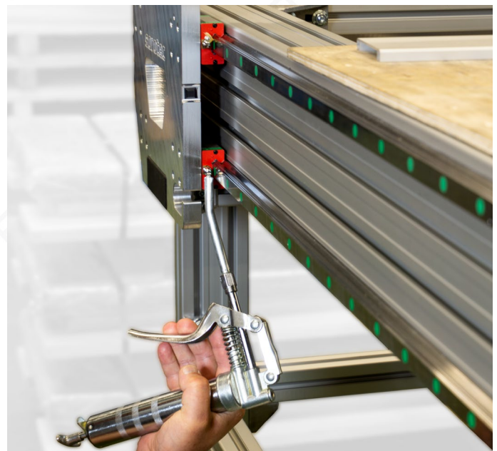
Fig. 2: Lubricating guide carriages X-axis
