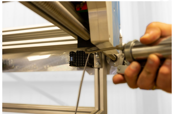
Fig. 4: Lubricating the right X spindle (gantry version)
