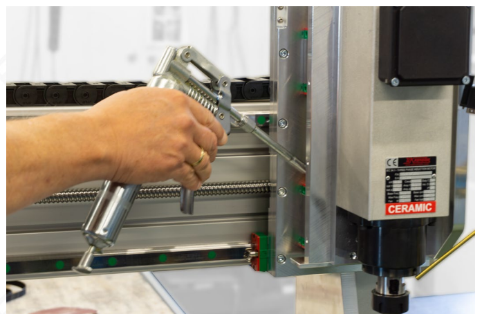
Fig. 8: Lubricating the left Z-guides
