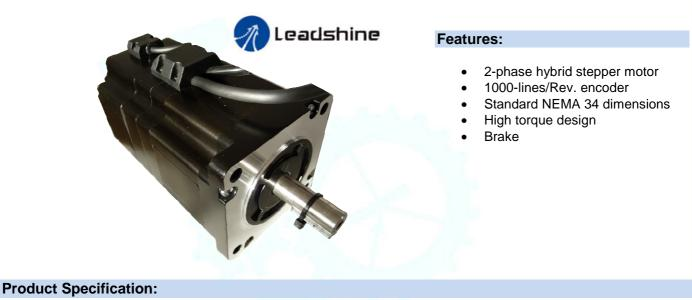
The CS-M23445B two-phase stepper motor with encoder feedback is designed to work with the Leadshine Hybrid Servo Drive CS-D808 or CS-D1008 to build a hybrid servo closed loop system (no loss of steps anymore). This version is additionally equipped with a brake that prevents the motor from rotating without active power supply.
