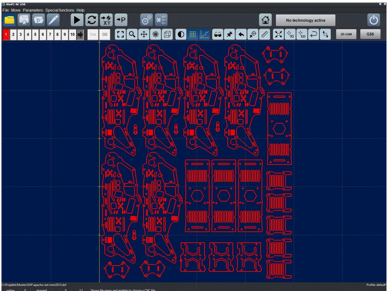
CAM-Functions : Loaded DXF-file with larger quantity and many contours
