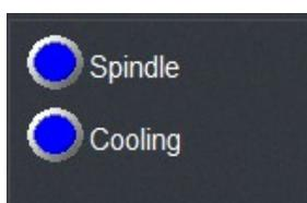
These spindle and coolant check boxes control their respective functions during jogging.
