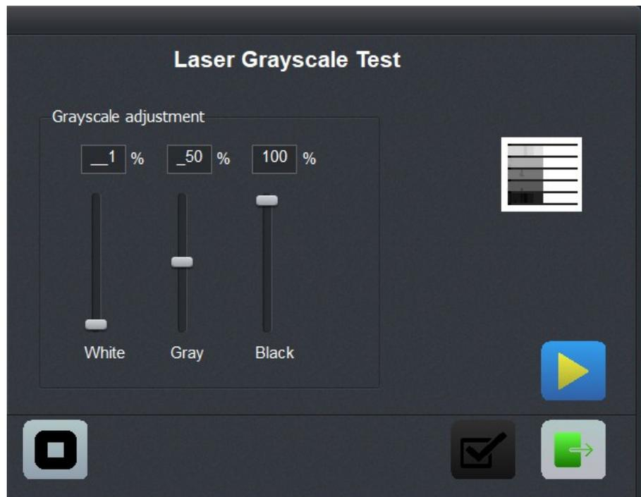
Part 2: Determining grey scaling with three support points
