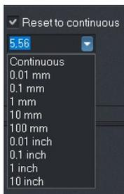
The discrete distance may be entered or selected from the pop up menu. The size and units of the menu distances are determined by the units setting in parameters (Metric or Imperial).
