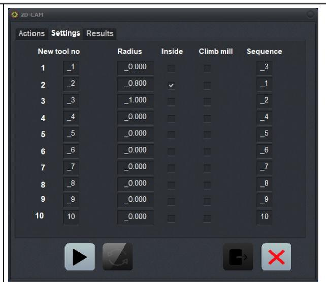
2. We define the values for tools 2+3, and start a search for contours, calculate radius compensation, and optimize any empty moves. The result is...
