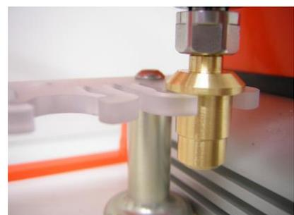
Correct the X- and Y-position in order for the greater diameter to dip into the exact center of the magazine without bending it in any direction.
