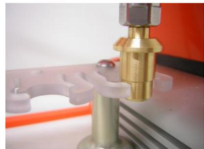
Move the calibration pin in the manual mode barely above the tool pocket 1 (far right in the magazine), as shown in the picture.
