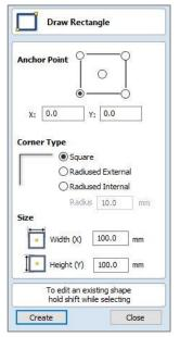
To draw the outer contour of the square, open the tool **Create Vectors / Draw Retangle**. As the anchor point is at the buttom left (workpiece zero point), the value for X and Y has to be 0. The width (X) and height (Y) are identical with each 100 mm.
