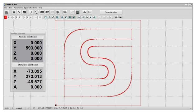
On closer inspection of the circular arcs, you will see that the circular arcs are created out of a multitude of single aligned arcs.
