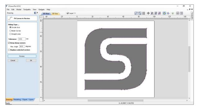
With the default settings, circular arc with a 0,01 mm tolerance, you will receive a good result. The parameters can also be set differently. Via the preview function you can directly see the adjusted settings.
