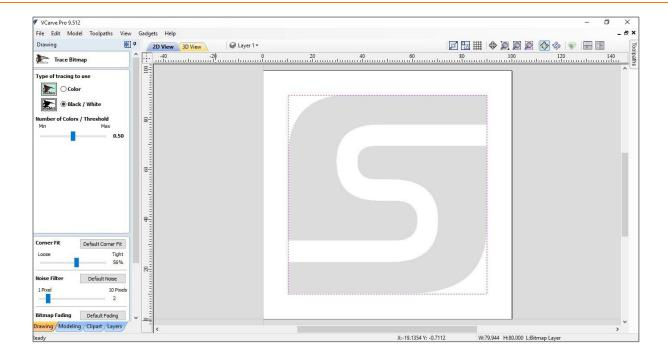
As type of tracing select black / white. Leave all other settings, e. g. corner fit and noise filter, at the default values. View the result of the vectorization via the preview button. By clicking **Apply** the illustration is converted into vectors.
