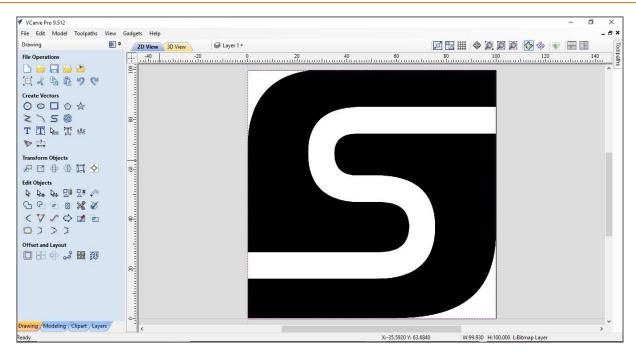
Select the imported logo by clicking the left mouse button, select the scaling tool (left side of the screen) via **Transform Objects / Set Selected Object Size** and enter 80 mm as width / height. Confirm the entry via clicking **Apply**.
