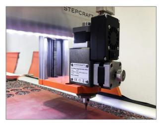
Connect the controller of the OTK-3 to the system output of your STEPCRAFT CNC system using the supplied 15-pin D-Sub connection cable. Make sure the blade cannot crush or cut the cable while the machine is moving.
