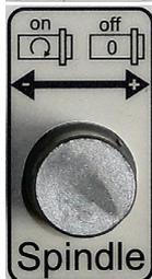
In manual mode, the activation of this button will start or stop the spindle. During a running job, the spindle speed can be regulated from 10 % to 200 % of programmed speed. Activating the button will stop the spindle and reset the speed value to 100 %.
