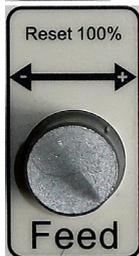
Rotation of the knob will immediately regulate the feed rate between 10 % and 200 % of the programmed value. By pushing the button, the feed rate will reset to 100 %.
