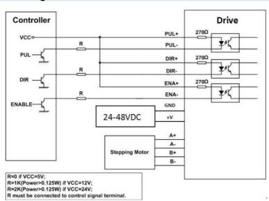
A complete system consists of stepper motor, stepper motor driver, power supply and controller (pulse generator). A typical connection diagram is shown in the left figure.
