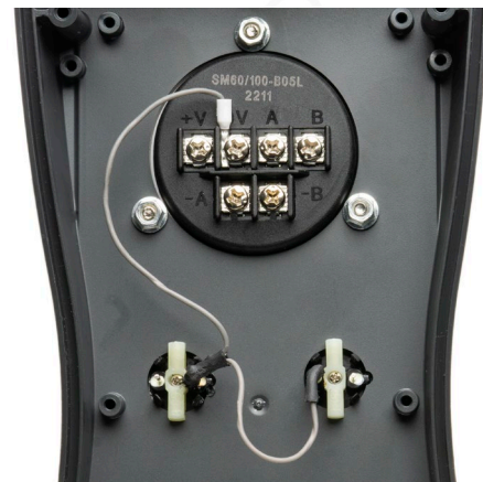
9 Ground connection of rotary encoder and buttons
