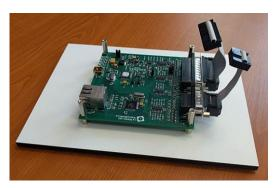
Step 6. Mount the breakout board and fix the board with the four M3 screws....and connect both cables...
