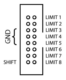
LIMIT 1-8 connects limit switches. It's recommended that a 100nF capacitor is connected directly across switch terminals.
