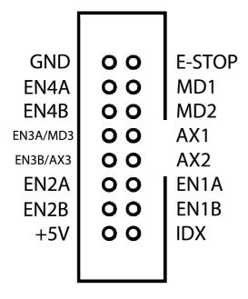
This connector provides inputs for use of MPG pendant devices and E-Stop. Spindle speed encoder for spindle synchronization can also be connected. GND pin provides 'Ground' or common connections.
