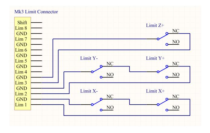
Serial wiring of NC type limit switches\* using Planet-CNC 16-pin adapter board:
