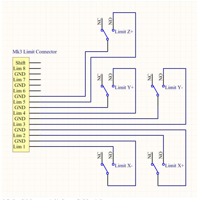
Each limit switch is connected to its own limit input pin.
