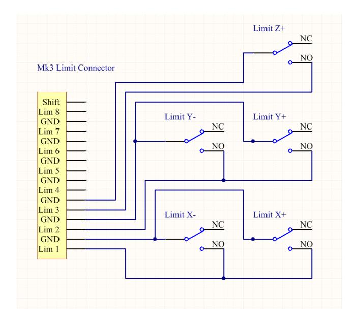
Parallel wiring of NO type limit switches\* using Planet-CNC 16-pin adapter board:
