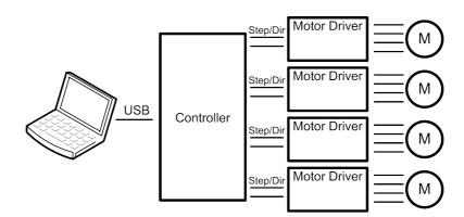
The PlanetCNC series of USB CNC motion controllers is link between a personal computer and motor drivers supporting step/direction control. PlanetCNC series of motion controllers are compatible with most motor drivers. The controllers use the USB port, available on all modern computers and laptops. They can serve as direct replacement or upgrade for many parallel port break-out boards. There are different models available.
