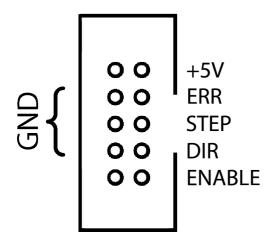
Each connector controls one motor driver. Controller has 9 connectors for axes 1-9. This means 9 axes which can all be moved at same time.
