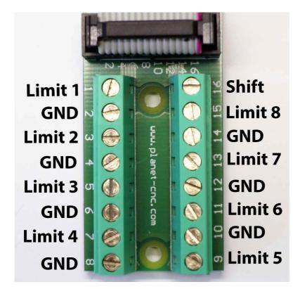
Bellow are wiring plans and pictures that demonstrate wiring of limit switches when 'Normal' or 'Single input' method is used.
