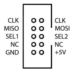
Connector for additional IO extension boards.
