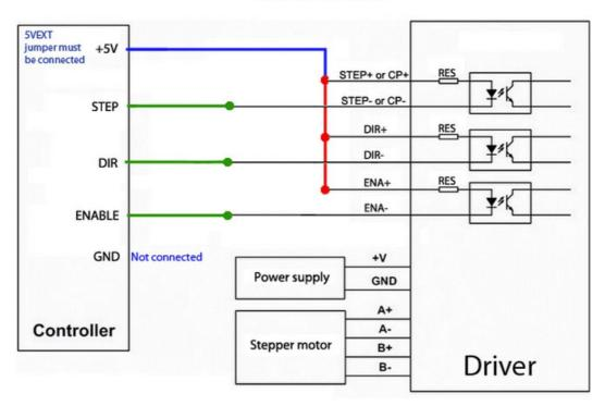
\*STEP input on motor drivers can be also labeled as PUL or CLK.
