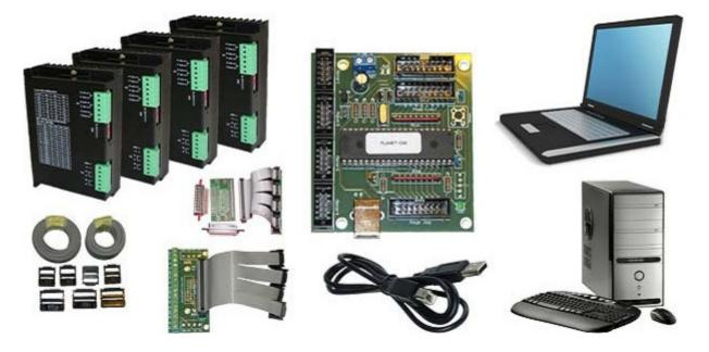
Installation of PlanetCNC CNC USB Controller requires a USB equipped PC or laptop along with motor drivers appropriate to the motors in use. The USB CNC controller is compatible with the vast majority of motor drivers that use step/direction signals.
