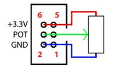
A potentiometer attached to this connector provides a manual jog speed control when using jogging keyboard connected to *JOG* connector. Mk3 controller also has this pins on jogging connector.
