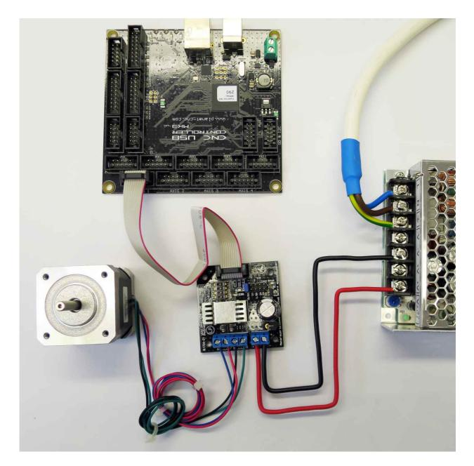
Picture bellow demonstrates connection of motor driver to Mk2 controller with screw type adapter and connection of controllers external power supply:
