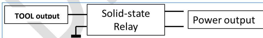
Figure 5. Connecting a solid-state relay.
