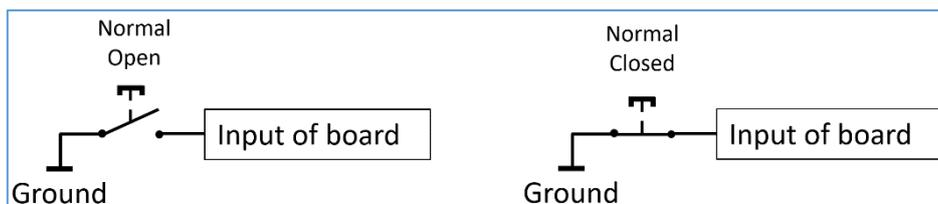
Figure 15. Connecting switch to E-STOP input.
