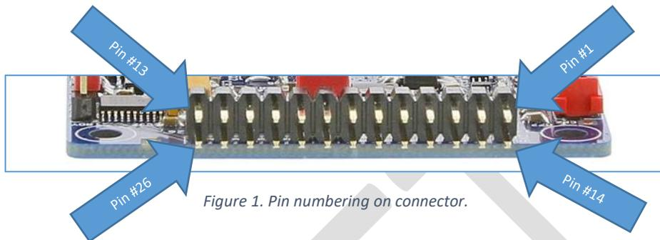
Figure 1. Pin numbering on connector.
