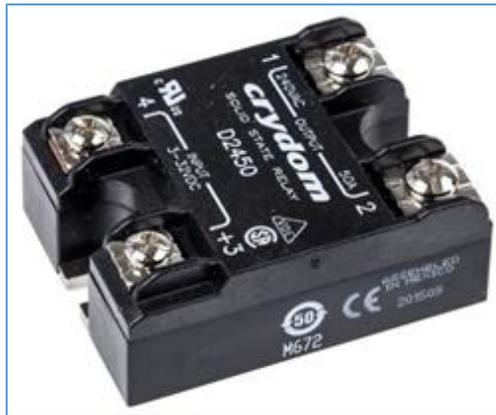
Figure 4. Example of solid-state relay.
