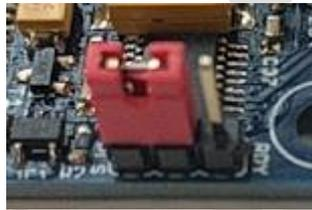
Figure 10. Output is square wave if SYSREADY is active.
