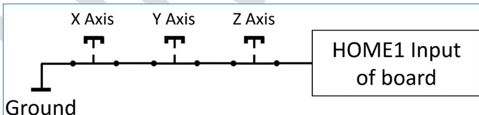
Figure 17. Connecting Normal-Closed home switches in series.
