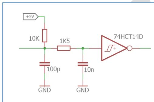
Figure 11. Probe input circuit.
