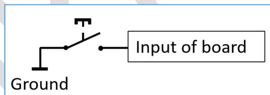
Figure 12. Connecting switch to probe input.
