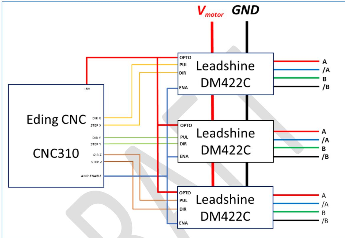
Figure 21. Connecting CNC310 to Leadshine DM422C.
