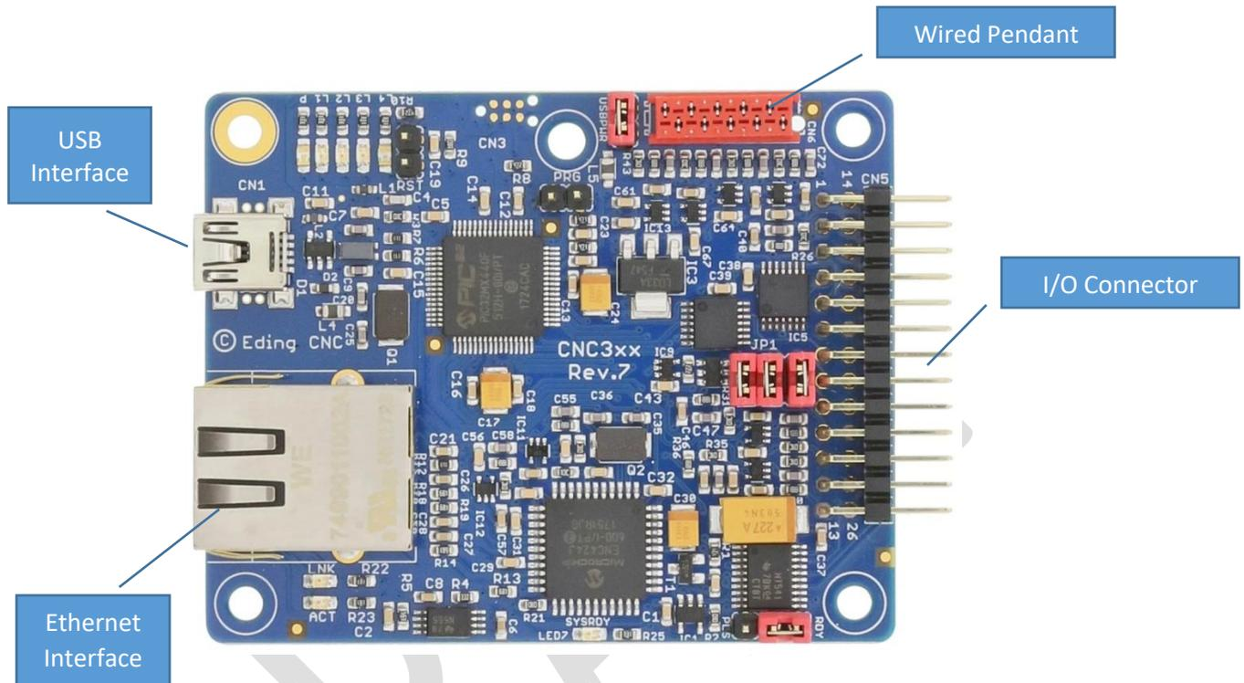
The purpose of the board is to offer a simple controller that can be used for operating small CNC machines that need only limited I/O.
