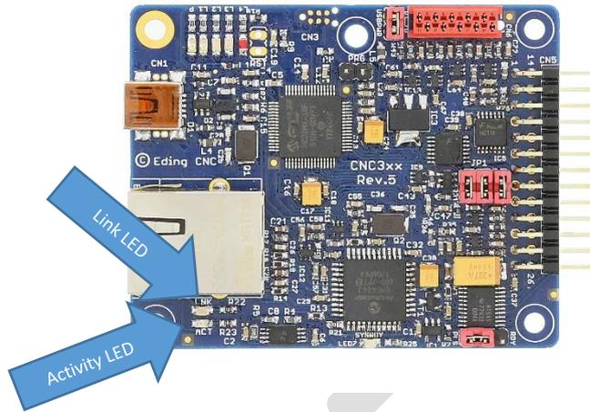
The LINK LED indicates if a network cable is connected. The ACTIVITY LED will blink if there is network communication.
