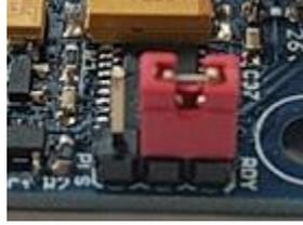
Figure 9. Output is HIGH if SYSREADY is active
