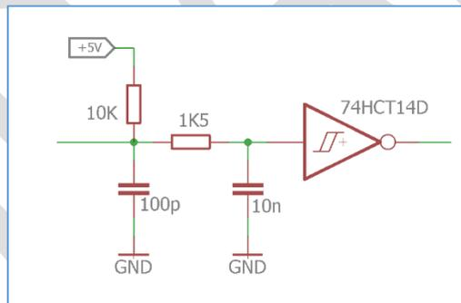
Figure 14. E-STOP input circuit.
