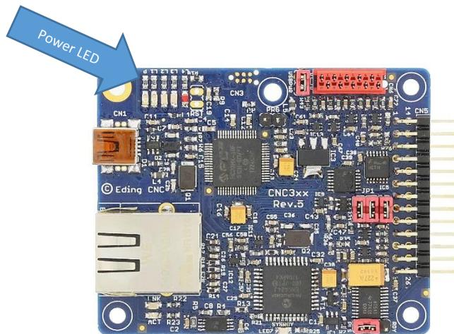
This blue power led indicates when power is applied to the board.
