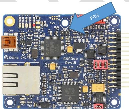
If this jumper is placed the board will skip the bootloader mode and will go directly to starting the firmware.
