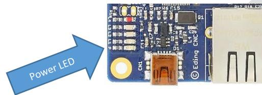
*Step 3.* The board is now able to communicate with the application software. If you startup the software the board should be found. This is indicated by the controller type 'CNC310' appearing in the top-left of the window. If the board is not found it will show 'SIMULATION'.
