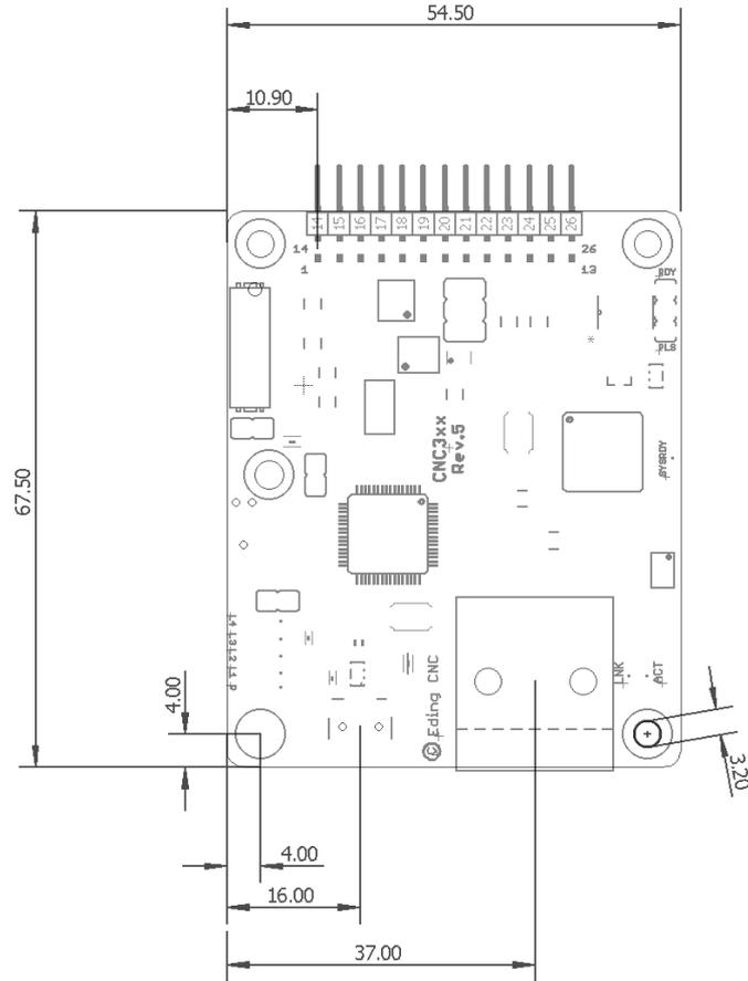
The controller can simply be connected by using standard connector (2x13 pole), pitch 2.54mm/0.1”:
