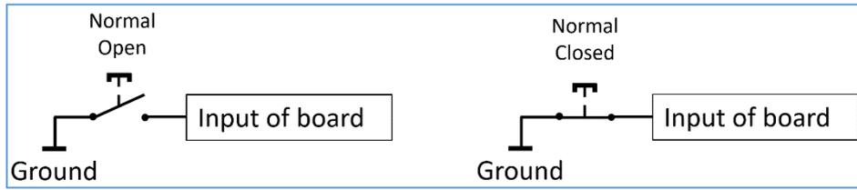
Figure 20. Connecting switch to HOME4 input.
