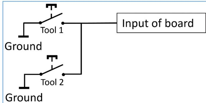
Figure 13. Connecting multiple tools to probe input.
