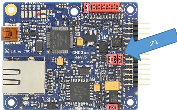
This jumper can be used to deactivate the signals on some I/O pins. Currently make sure that all jumpers are mounted.
