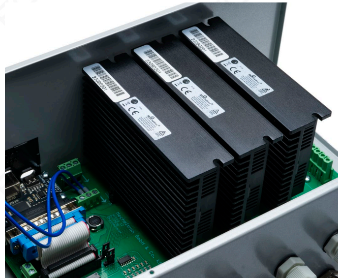
Fig. 20: Attached power amplifiers
