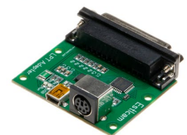
Image 9: Board with adapter module, here for Benezan / Beamicon. In front a module for Estlcam for comparison.
