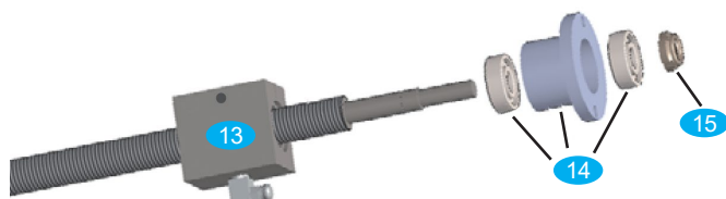
Fig. 1: Assembly of the ball screw
