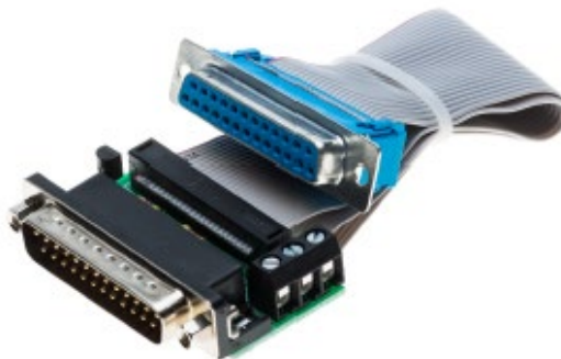
Fig. 6: Adapter board with connection cable
