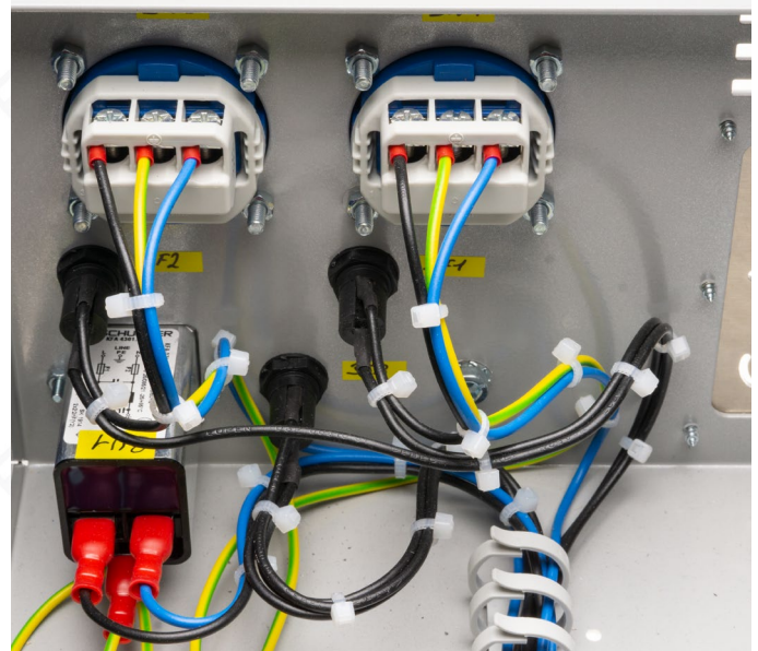
Fig. 13: Sockets for cooling and milling spindle, fuse protection, built-in plug with line filter
