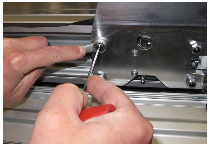
Fig. 21: Adjusting the guide rollers
