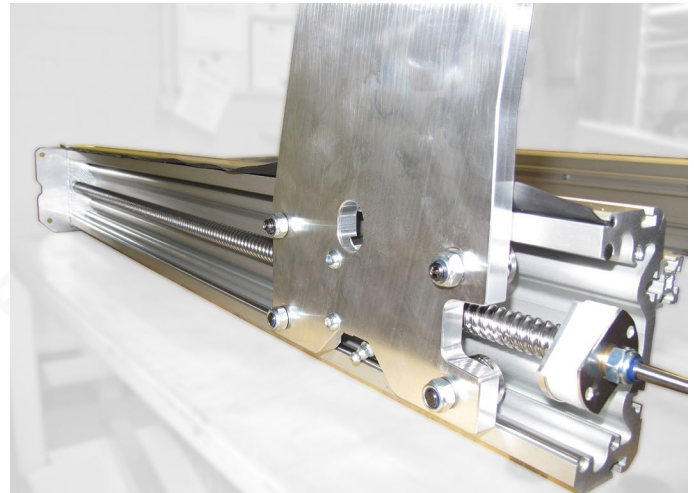
Fig.17: Installation of the right portal cheek
