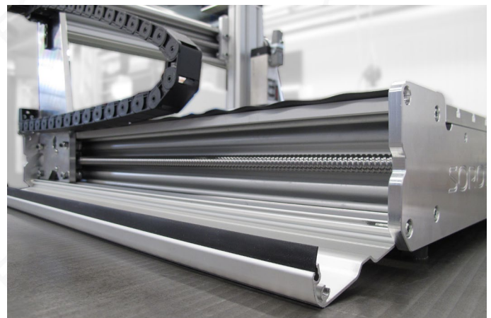
Fig. 28: For maintenance of the spindles, the side covers can be easily opened after removing the upper screws.
