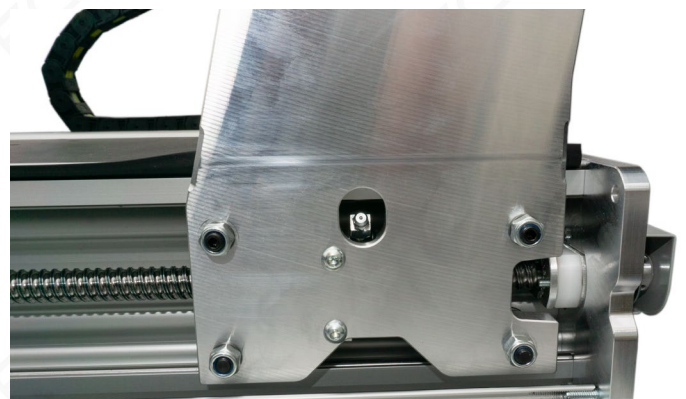
Fig. 12: Right portal cheek with nipple through hole.
