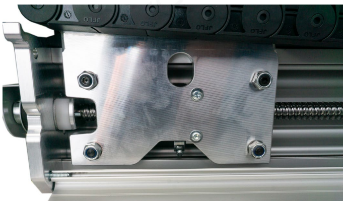
Fig. 11: Left portal cheek with nipple below.
