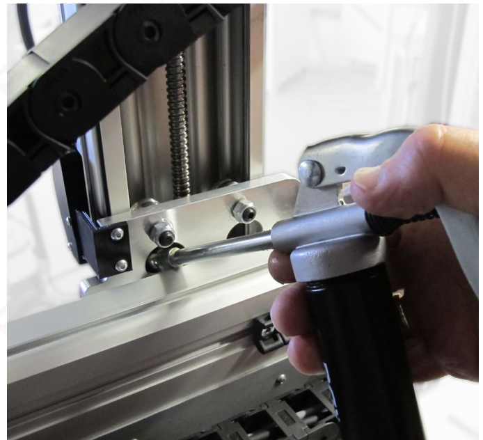
Fig. 47: Lubricating the Z axis
