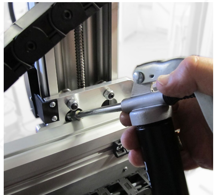
Fig. 47: Lubricating the Z axis
