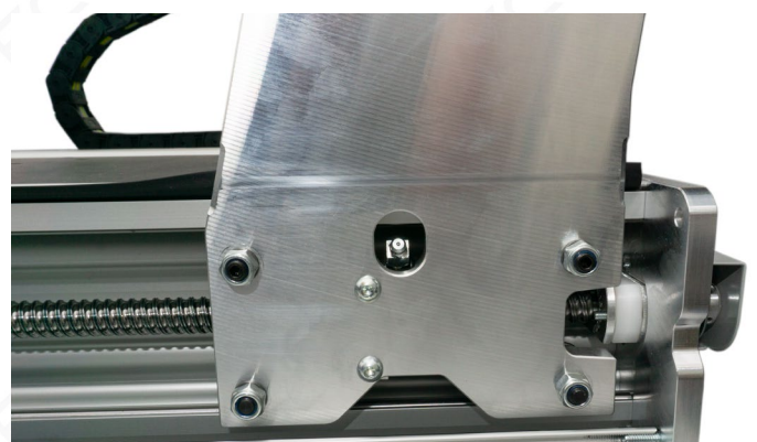
Fig. 12: Right portal cheek with nipple through hole.
