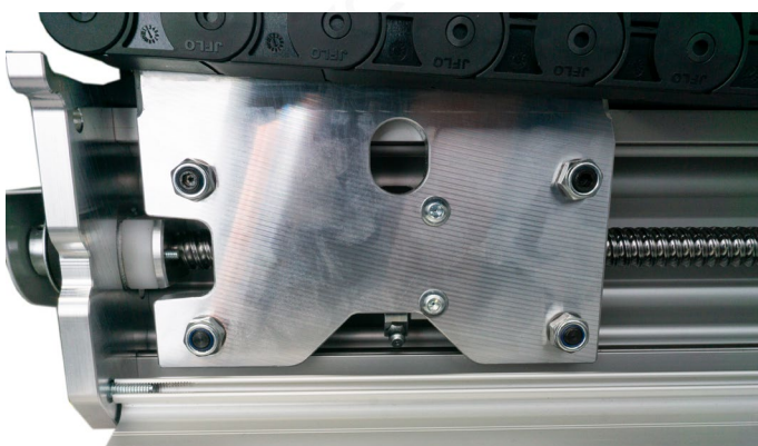
Fig. 11: Left portal cheek with nipple below.
