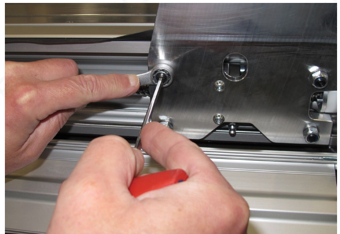
Fig. 21: Adjusting the guide rollers
