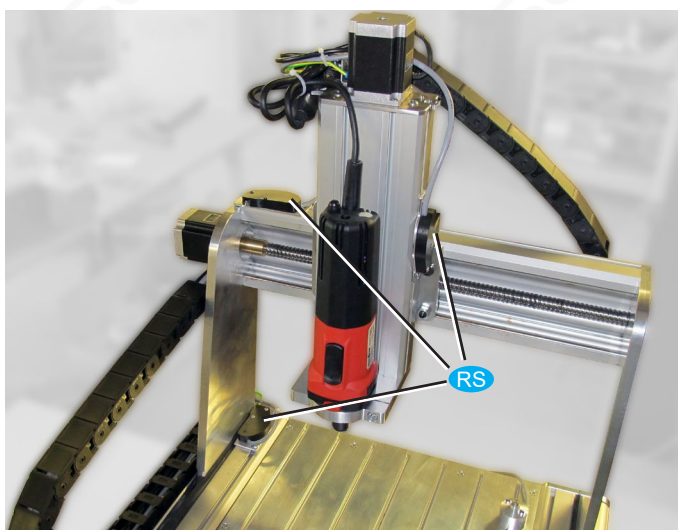
Fig. 30: Position of the reference switches on the machine
