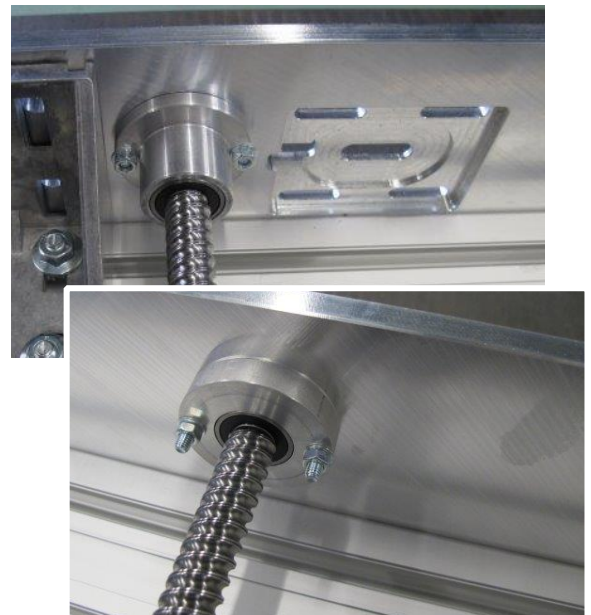
Fixed bearing (above) and floating bearing in a Sorotec Alu-Line
