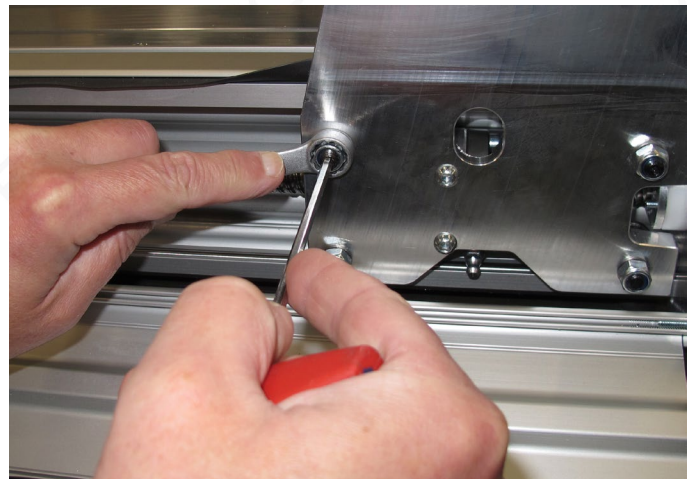
Fig. 21: Adjusting the guide rollers
