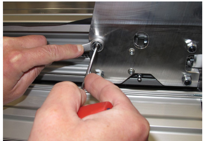
Fig. 21: Adjusting the guide rollers
