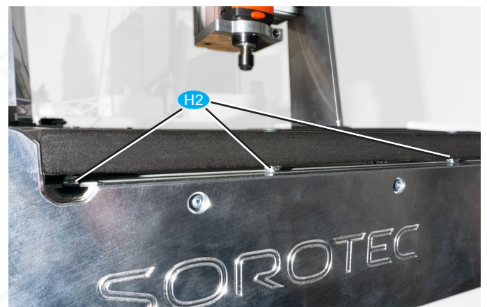
Fig. 42: Hammer nuts not yet properly aligned
