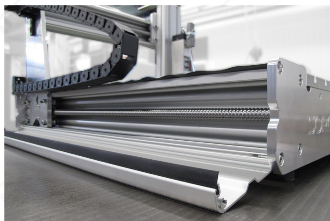
Fig. 28: For maintenance of the spindles, the side covers can be easily opened after removing the upper screws.
