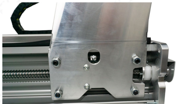
Fig. 12: Right portal cheek with nipple through hole.
