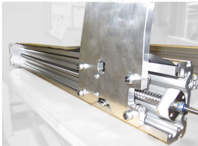
Fig.17: Installation of the right portal cheek
