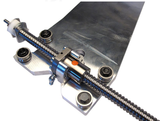
Fig. 10: Right portal cheek with mounted spindle.
