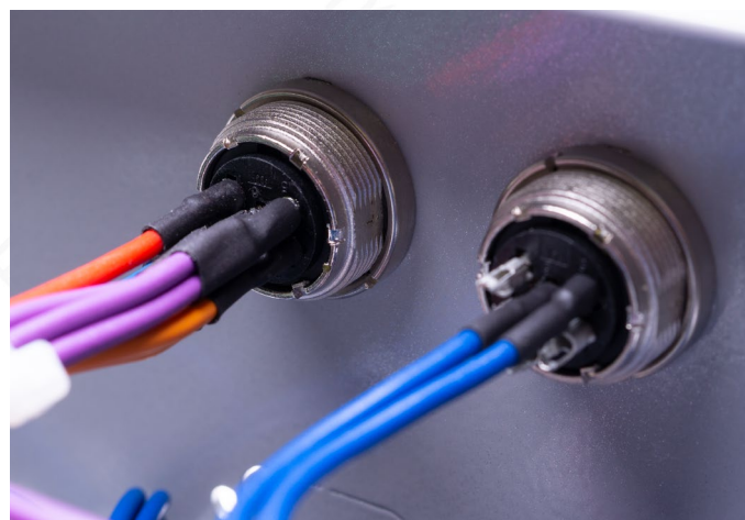
Fig. 17: Each pin individually insulated with shrink tubing
