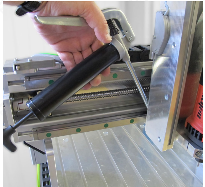
Fig. 46: Lubricating Y-axis carriage
