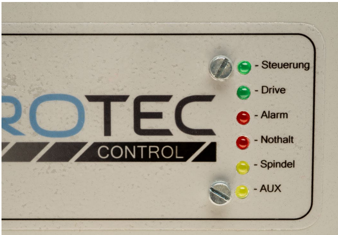
Fig. 31: Status LEDs show the operating status
